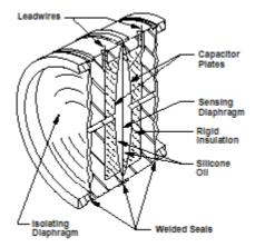
An electronic-type transmitter is shown in the figure above. This particular type utilizes a two-wire capacitance technique.
