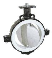
Butterfly values have a lever that allows the operator to open or close the value to control the flow. These values are part of a family known as rotary values, which are defined by the quarter turn that is used to move from the open to closed position and vice versa. This results in a lower surface friction, which means that these values can be smaller than others and still operate efficiently.
