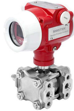
MDMP305X-DST Industry Std Differential (gage, abs) Pressure Transmitter Measuring Range: 200 Pa~10 MPa Accuracy:±0.075 % URL (옵션 ±0.05% URL) Output: 4-20 mA, HART, Fieldbus
